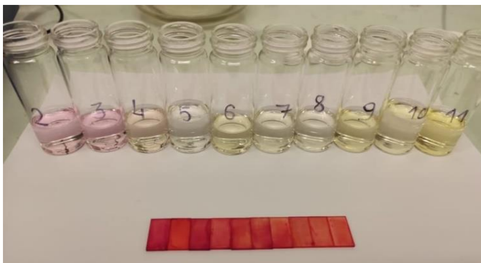
Figure 1. Test plates coated with sensor films after 3 days in solutions with pH values 2-11
